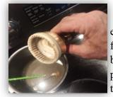
Next, you prep the parts. As with anything else, the better the prep, the better the results. I found sanding with 800-grit, then cleaning with brake-cleaner to be satisfactory for this previously plated brass housing. After cleaning, I masked the threaded and interior sections with some warm
